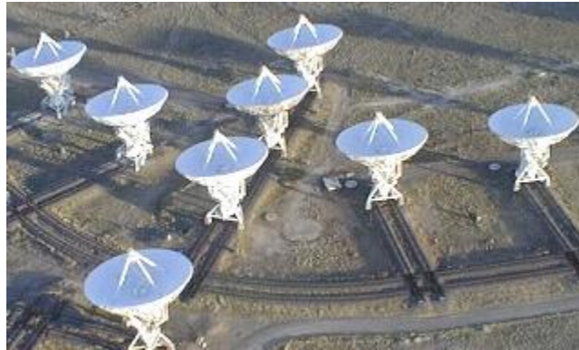
Figure 4.4 The Very Large Array (VLA) near Socorro, New Mexico, is an example of interferometry. The 27 dishes are arranged in a “y”-shape in conjugation with the rotation of the earth to create what can be thought of as one very large radio telescope. 22
